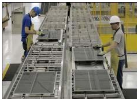
Panels are trimmed at First Solar's Perrysburg Township plant, the firm's only U.S. factory.
